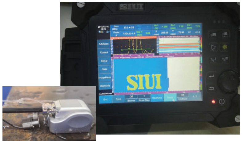
DLA detection for 8mm plate
