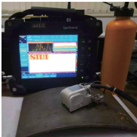
DLA detection for curved panel
